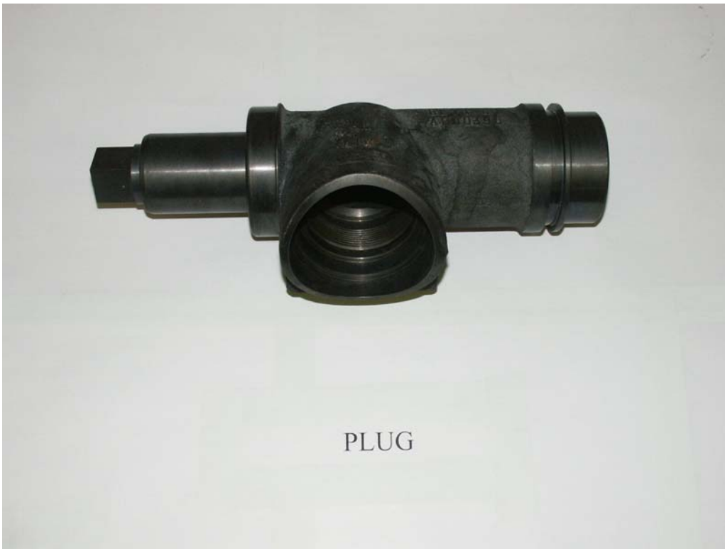
PLUG (Index mark can be found on the stem flat that faces the same way as the plug seal opening.)
